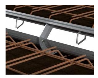
6. Fasten the E-Z Mount Brackets at each U-drain bracket interval, using the hardware supplied. Pound appropriate lengths of rebar into your base material with the rebar running through the conduit portion of the E-Z Mount Bracket. Make sure that all section tops are level. When the correct levels are achieved, tighten the set bolts on the E-Z Mount Brackets to secure the U-Drain.
