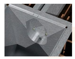
5. Bolt all remaining sections of U-drain together using the lettered flanges as a guide. Loosely tighten bolts until full length of drain is installed. Ensure that the drain run is straight and make adjustments as neccessary. Tigthen the bolts.
