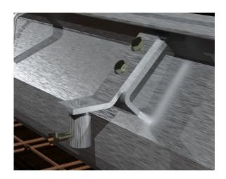
4. Bolt the last section of U-drain (deepest) to the sump pit. If there is a pre-existing sump pit or no pit at all, install the deepest U-drain section against the forming.
