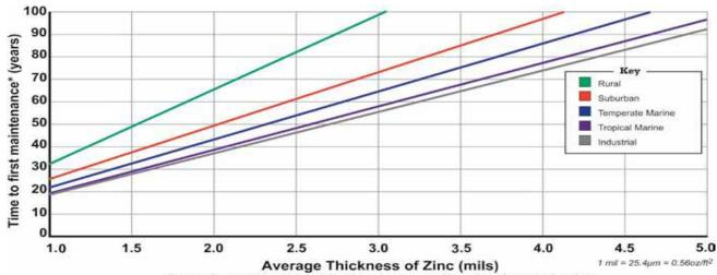
\*Time to first maintenance is defined as the time to 5% rusting of the steel surface.
